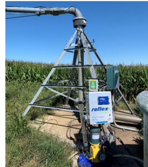
Figure 4. Center pivot system equipped with a variable injection rate fertilizer pump.
