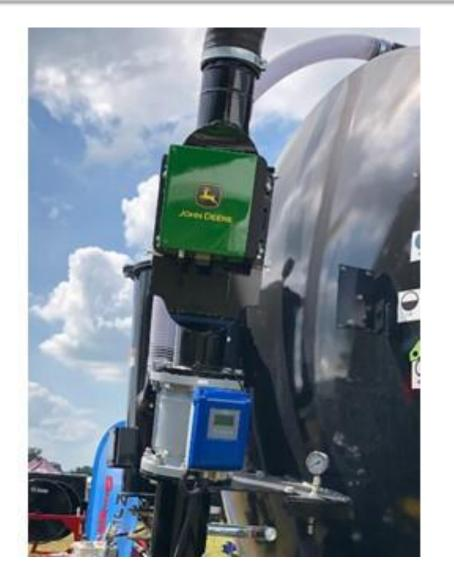
John Deere manure nutrient sensor (top) combined with flow meter (bottom).
